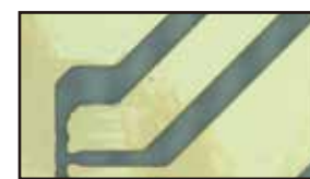
炉前锡球 Pre reflow solder ball
