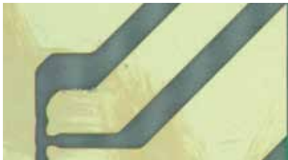
炉前锡球 Pre-reflow solder ball
