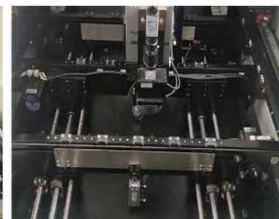
单头双轨设备 Single-head Dual-track Equipment
