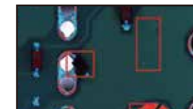
沾锡 Excess solder
