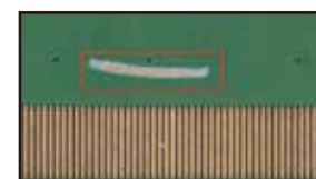
漏铜 Copper Leakage
