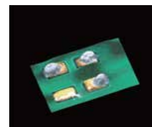
漏印 Print leakage
