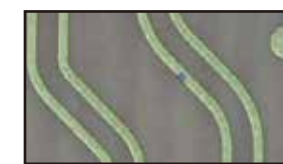
沾锡 Excess solder
