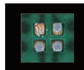
少锡 Insufficient solder
