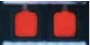
漏印 Print leakage
