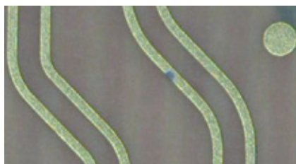
沾锡 Excess solder
