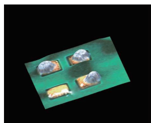
漏印 Print leakage
